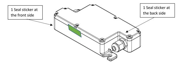
In the case that is needed to break a seal to access the S1 switch (e.g.: for adjust the scale after a calibration), please consult your representative, because an official re-verification of the weighing instrument could be mandatory depending on legal regulations in your country.
